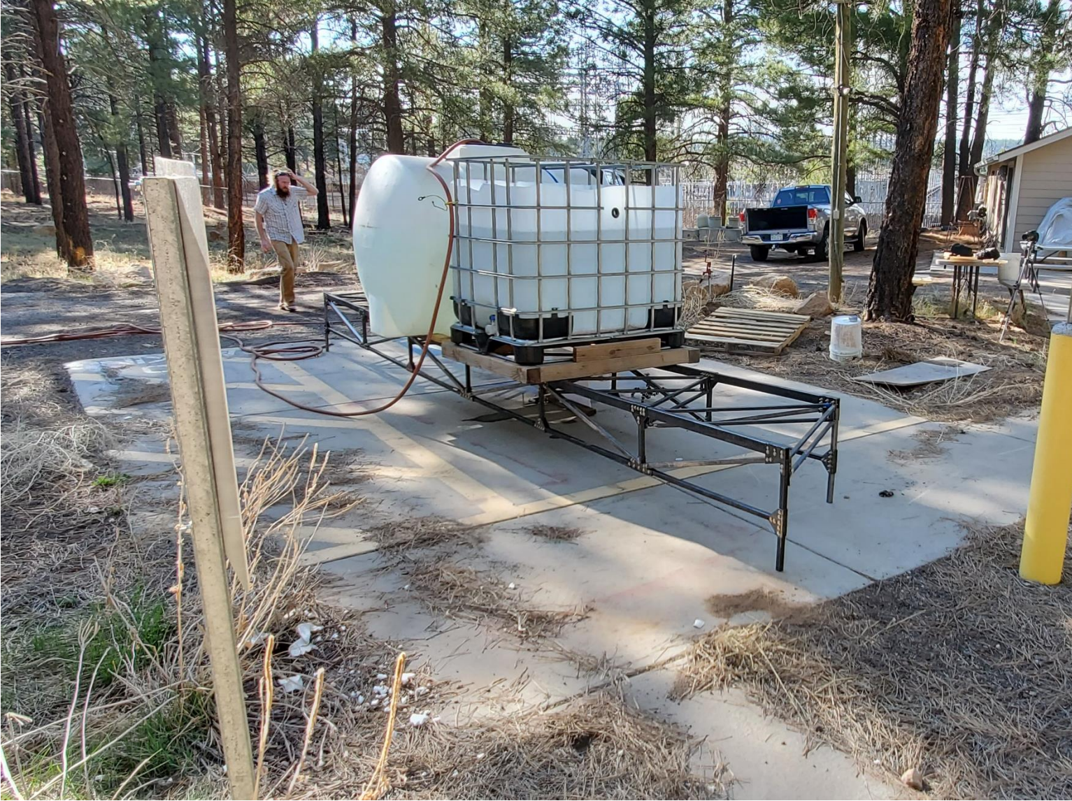
Figure 3: Loading of bridge with water
