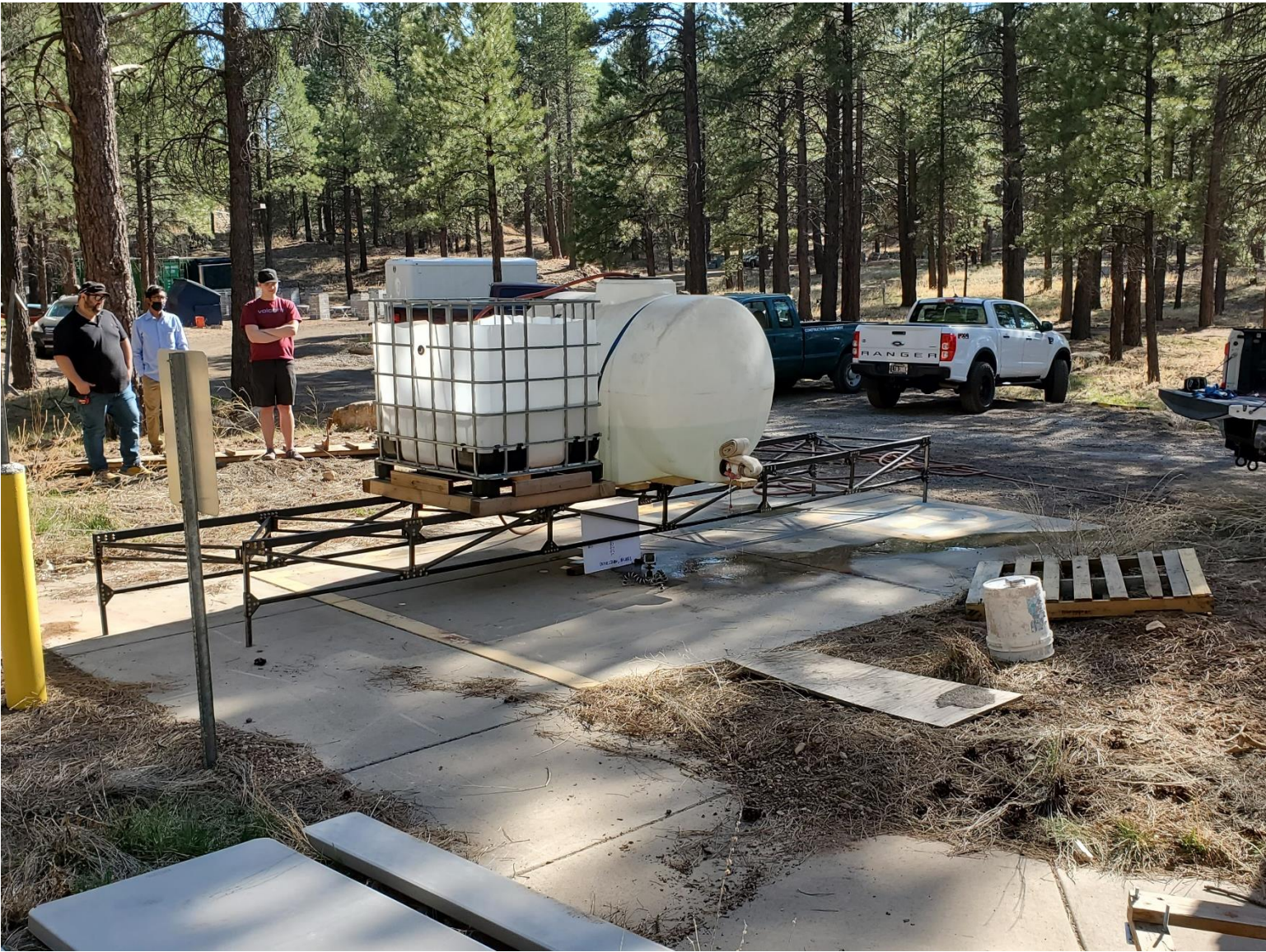
Figure 2: Early stage of loading bridge with water
